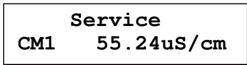
The first line of the LCD display shows the actual situation (phase) of the installation.
