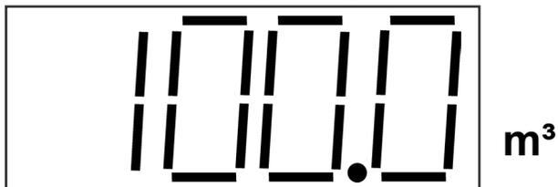
Whilst a unit is in service the LED - display indicates the remaining volume of water which can be softened before the next regeneration will be required.
